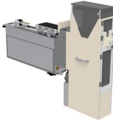
The FEEDER-TRAY module is used to feed the components into the machine from Jedec Trays. It consists of the actual module and the upstream Traylift, that can be separated from the module, in which both the full and the empty trays are deposited. Full trays are fed individually to the module, positioned for removal of the individual components and transported back to the Traylift as empty trays.
