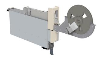
The TAPE-FEEDER module is used to feed the components into the machine from blister tapes. It consists of the actual module and the upstream reel from which a full blister tape is unreeled in each case and fed to the module. The cover tape is removed there from the blister tape to allow removal of the individual components from the blister tape.
