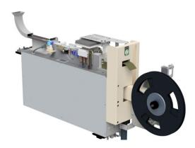
The tape module TAPER-NTP serves to package components in blister tapes. Placing the individual components in the blister tape is first followed by an optional placement check using a camera system, the tape transport and then sealing of the blister tape with a cover tape and winding of the tape. Tape modules for different tape widths are available, which can also be combined in a single machine, if necessary.
